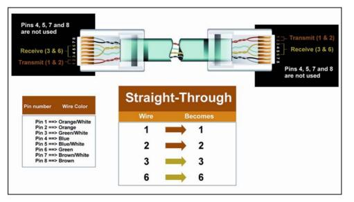
Figure4-1: Diagram of Straight Through Cables
